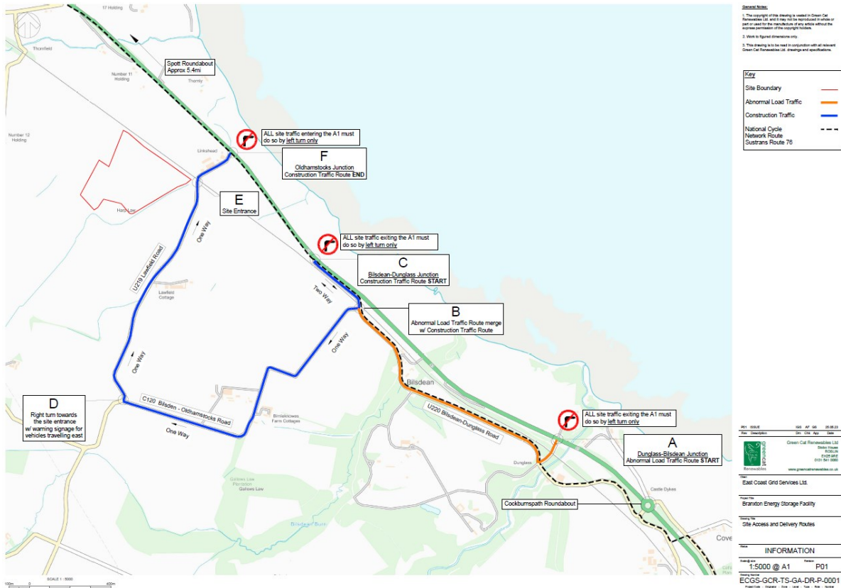
Figure 2.1 – Abnormal Load Delivery Route
